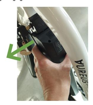
The battery can be removed from the frame for recharging. To remove the battery, turn the key (unlock) and pull the battery to the left by its upper end. BE CAREFUL OF ITS WEIGHT.
