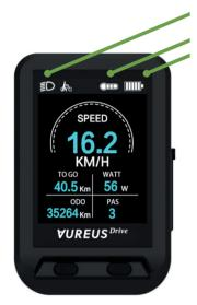
Lights on Engine temperature Battery charge level
