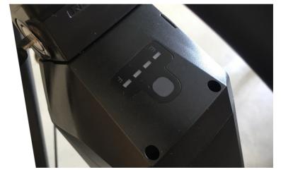
The battery can be removed from the frame for recharging. To remove the battery, turn the key and pull the battery to the left by its upper end. BE CAREFUL OF ITS WEIGHT.
